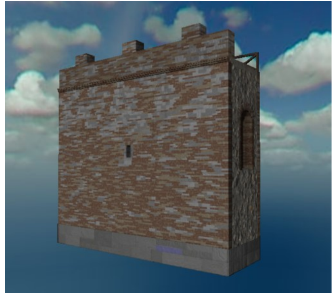
Figure 8: Screenshot of ATON with the photorealistic representation of the M2 portion. The user can freely investigate the model. Representing a single portion also makes it possible to observe the internal construction techniques and the presence of the covered walkway. (Nicola Delbarba).
