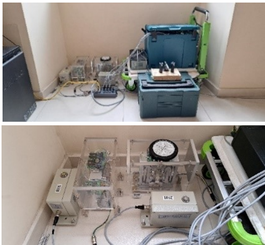
Figure 3. Monitoring system set-up: (top) 4 seismometers and 1 microphone; (bottom) detail of the 4 seismometers.
