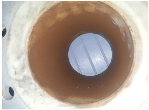
Figure 4. Inner pipe with encrustations.
