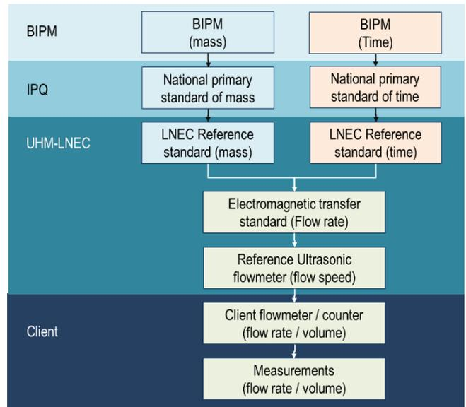
Figure 3. Traceability chain adapted to *in situ* calibration procedures of UHM-LNEC.
