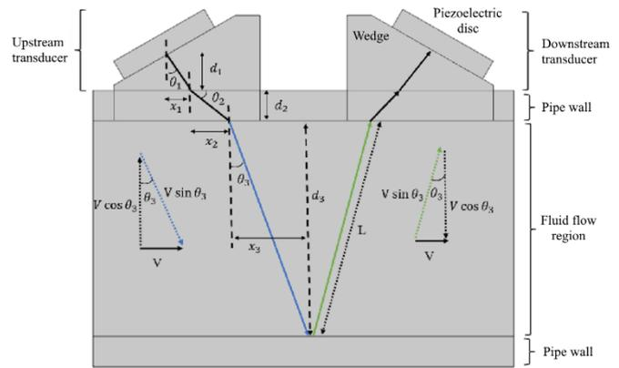
Figure 1. Schematic of the V-path method for Clamp-on ultrasonic flowmeters, adopted by [15].
