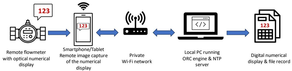
Figure 2. System implementation architecture.
