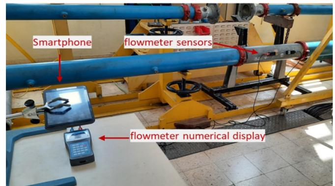
Figure 3. Experimental setup example for ultrasonic flowmeter calibration at the UHM-LNEC plant.
