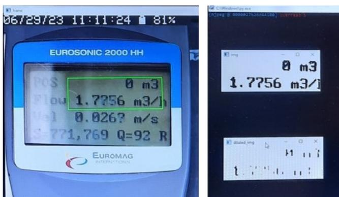
Figure 7. Left: Original image of the flowmeter numerical display with bounding box overlaid around the area of interest, Right: corresponding image converted in binary format.
