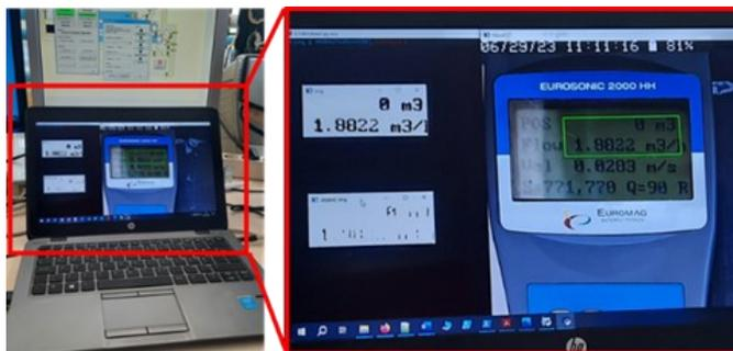
Figure 6. Remote image of the flowmeter display in the PC, in the monitoring and command room.
