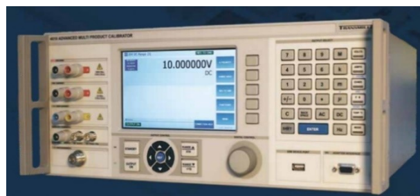
Figure 9. LEM reference standard - multifunctional calibrator Transmille 4015 with inductance calibration option.
