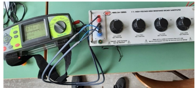
Figure 11. Testing set-up in LEM for calibration of Metrel MI 2077 TeraOhm 5kV with the 5 kV IET Labs HRRSQ resistance reference standards decade.
