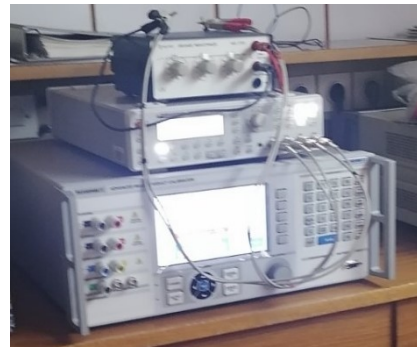
Figure 10. Testing set-up in LEM for calibration of ROHDE & SCHWARZ HM8118 LCR-Bridge with the Transmille 4015 Multifunctional Calibrator.
