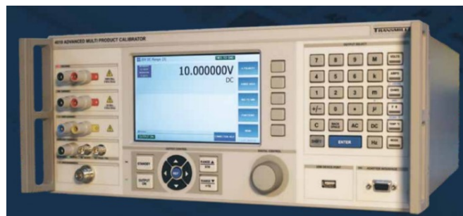
Figure 5. LEM reference standard - multifunctional calibrator Transmille 4015 with oscilloscope calibration option SPC600.
