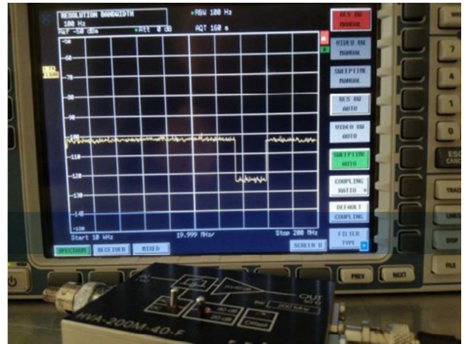
Figure 6. An essential setup for checking the parameters of components included in the measurement system, consisting of a spectrum analyzer, an amplifier -with known parameters, including equivalent voltage and current of input noise and frequency characteristics, and a source of white noise.
