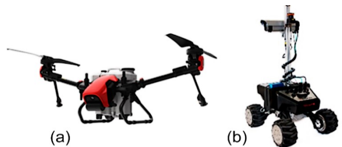
Figure 4. Two examples of commercial drones for agriculture. (a) XAG V40 drone with a 15 liters tank. (b) VINBOT an all-terrain autonomous mobile robot with a set of sensors capable of capturing data about water status, production, vegetable development, etc..
