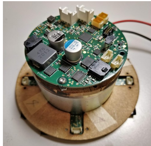
Figure 5. A simple prototype of the foot for electrical testing. The control board is placed on the top of the electro-permanent-magnet EPM. The image is adapted from [6].
