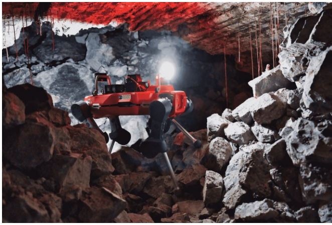
Figure 3. The climbing robot ANYmal operates in harsh environments [5].
