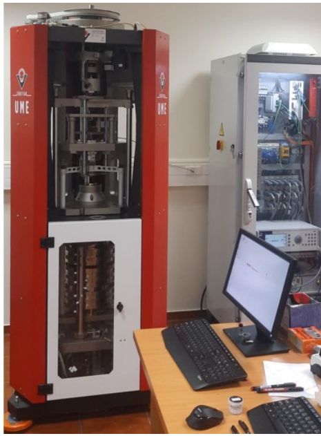
Figure 1. Rockwell-Brinell-Vickers hardness standard machine of TÜBİTAK UME.
