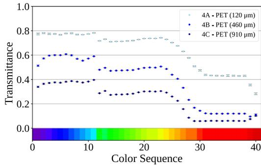
Figure 9. Transmittance of samples made with the same material and colour, but different thickness. The error bars represent the experimental measurement repeatability. Each point on the graph represents an individual measurement, with labels in the legend indicating the corresponding sample number and material type.
