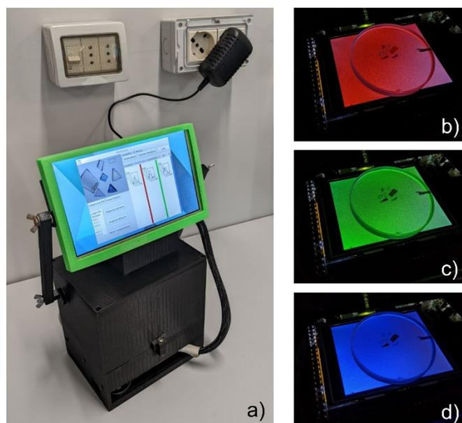
Figure 3. Photo of the developed measurement system. Inside the 3D-printed plastic box, the SUTs are arranged on the glass support above the LCD panel that illuminates the same SUTs with a pre-defined colour sequence, i.e., red (b), green (c), and blue (d).
