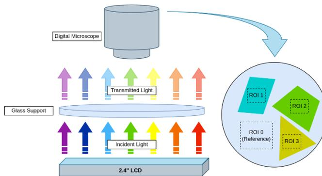
Figure 2. Measurement system schematic representation. The single-board computer UDOO is connected to the LCD Panel, surrounded by a transparent glass support, where the SUTs are placed. The light emitted by the LCD passes through the transparent glass support and consequently the samples and is captured by the USB digital microscope. From the acquired image, ROIs are selected to evaluate the transmittance value.
