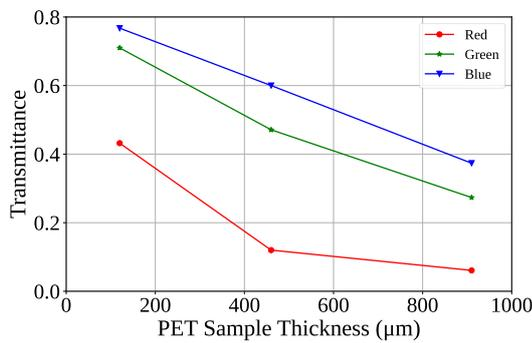
Figure 10. Transmittance as a function of the PET samples thickness at red, green, and blue colours.
