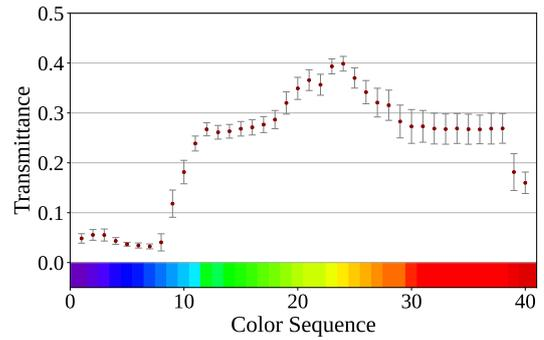
Figure 12. Transmittance of polyimide samples. Measurements were carried out on a total of 30 fragments derived from a commercial Kapton sheet with a nominal thickness of 127  $\mu\text{m}$ . The red points indicate the average transmittance value for each colour. The error bars represent the standard deviation.
