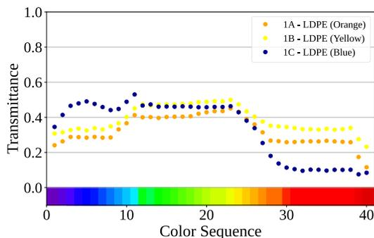
Figure 7. Transmittance of samples made with the same material and thickness, but different colours. Each point on the graph represents a single measurement, with labels in the legend indicating the corresponding sample number and material type.
