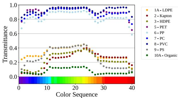
Figure 6. Transmittance of each type of material for the samples as a function of the colour sequence. Each point on the graph represents a single measurement, with labels in the legend indicating the corresponding sample number and material type.
