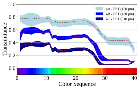
Figure 11. Transmittance of the samples made with the same material and colour, but different thickness. The bands represent the experimental measurement repeatability.
