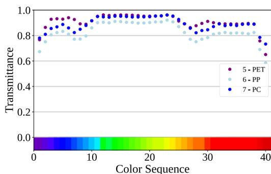
Figure 8. Transmittance of samples with the same colour and thickness, but different materials. Each point on the graph represents a single measurement, with labels in the legend indicating the corresponding sample number and material type.
