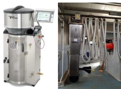
Figure 1. Vario Smart Förster-Technik feeder (left) and Calf Rail robotic arm (right).
