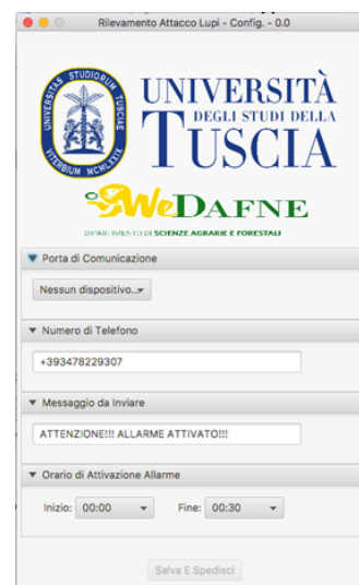
Figure 7. Application interface made to set the phone number to which to send alarm SMS messages and the operating time of the prototype.
