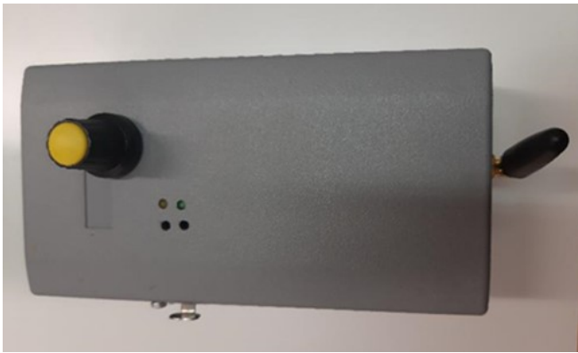
Figure 8. Detail of the prototype highlighting the acoustic detection threshold controller (potentiometer) and LED.
