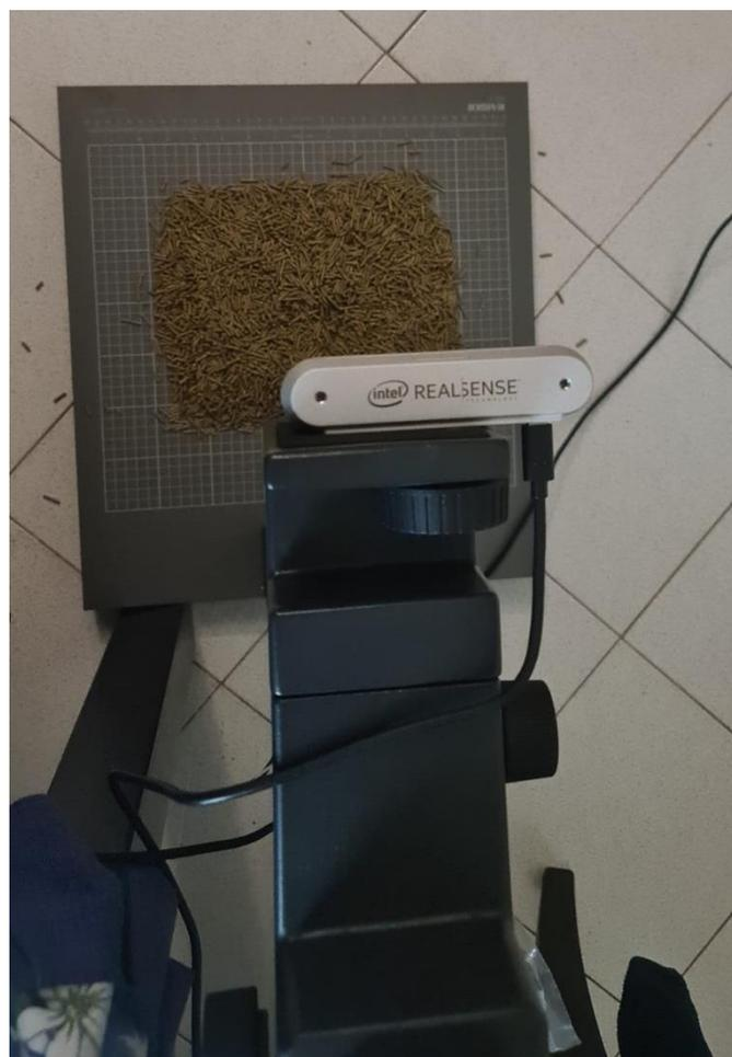
Figure 5. Realized setup for volume measurements of rabbit feed.
