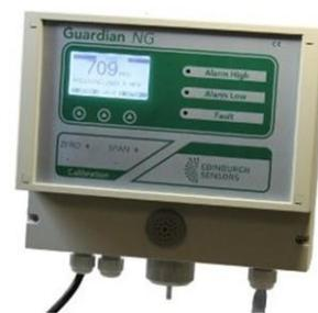
Figure 2 The Guardian NG CH<sub>4</sub> gas measurement system [41].
