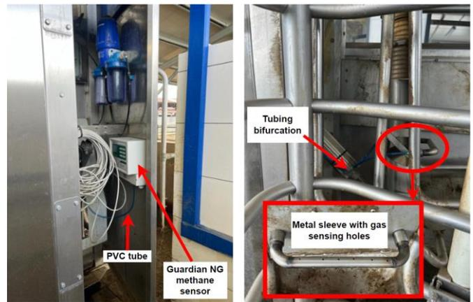
Figure 5. Field placement of the CH<sub>4</sub> gas emission sensing from ruminants.
