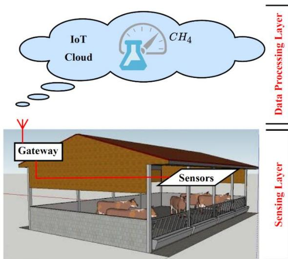
Figure 1. Generic scheme for Internet-of-Things based monitoring of enteric methane CH<sub>4</sub> emissions from ruminants.
