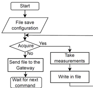
Figure 4. Flowchart example of the LabVIEW executing code.
