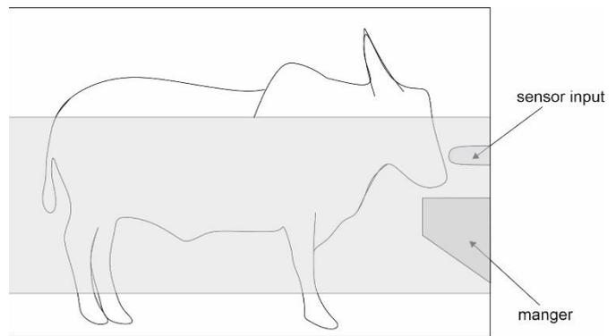
Figure 6. Drawing showing the field placement of the CH<sub>4</sub> gas emission sensor in the milking robot.
