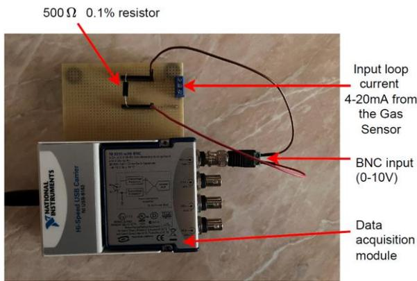
Figure 3. Scheme of the DAQ setup.
