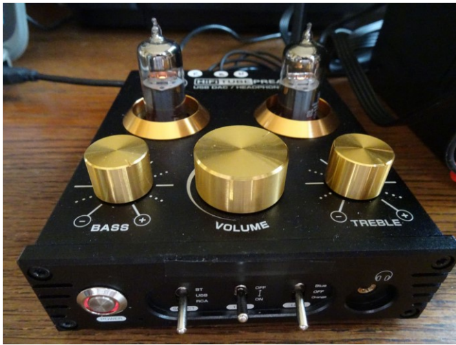
Figure 1. External view of preamp: front and top panel with vacuum tubes.
