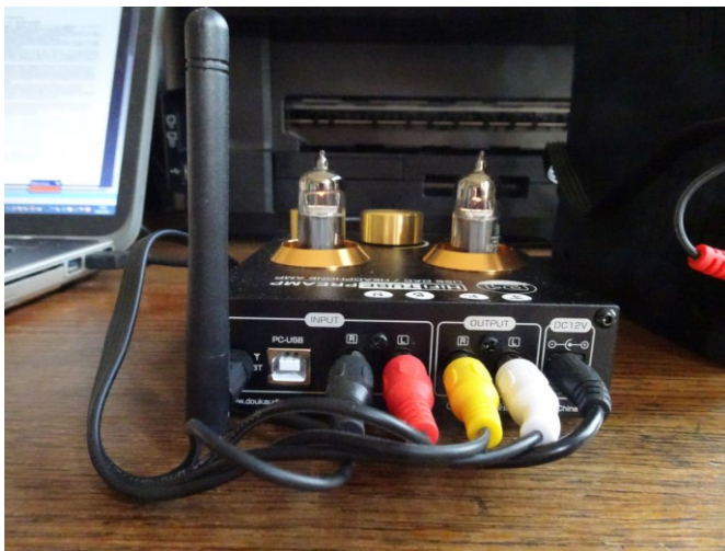
Figure 2. View of rear panel showing connectors and bluetooth antenna
