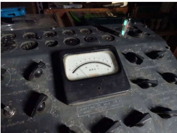
Figure 16. Experimental setup with tube tester Metrix 310B (EM84 indicator tube under test)
