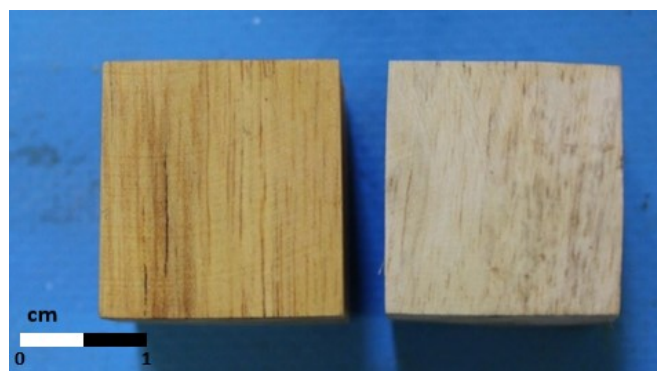
Figure 7. Comparison of wood specimens consolidated with Paraloid and subjected to artificial aging before (left) and after (right) cleaning with Hydrogel PVA-Borax loaded with Acetone and Ethanol in a 1:1 ratio.
