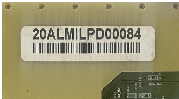
Figure 4. Label example on a PDB. Any PDB has a barcode that is a unique code.
