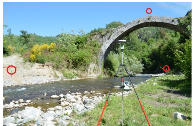
Figure 11. GNSS receiver on a TLS station point. Three targets, circled in red, are visible.
