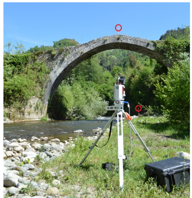
Figure 12. The TLS on a station point. Two targets, circled in red, are visible.
