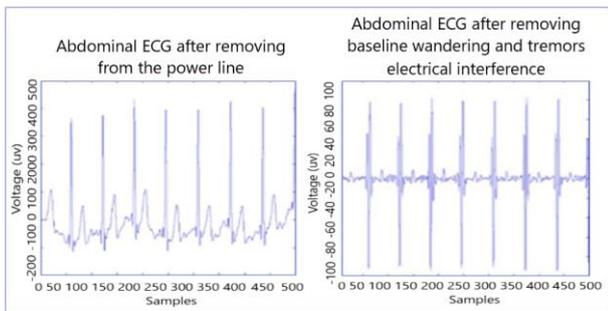
Figure 12. Abdominal ECG after suppressed power line interference noise at 50 Hz and Abdominal ECG after removing interference from the power line, line based on the wandering and trembling.
