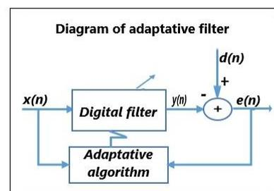
Figure 6. Diagram of adaptive filter.
