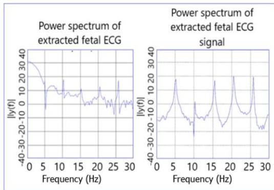
Figure 13. Power spectrum of simulated mother ECG signal and power spectrum extracted fetal ECG signal.
