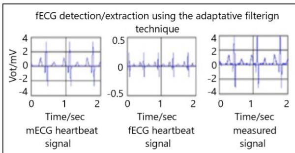
Figure 7. Fetal ECG detection/extraction using the adaptive filtering technique.
