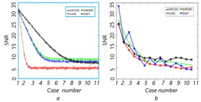
Figure 20. A comparison of the SNR of the MUSIC, MEMD, LMS and EWT algorithms for ECG (a) and apneas (b) of the mother and the fetus.
