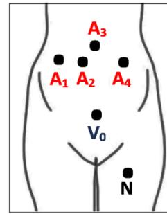
Figure 4. Acquisition of the maternal and fetal ECG signal,  $A_1 \dots A_4$ : abdominal leads,  $V_0$ : reference electrode,  $N$ : active ground.
