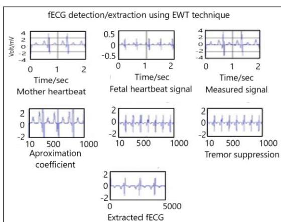
Figure 9. Fetal ECG detection/extracted using EWT technique.
