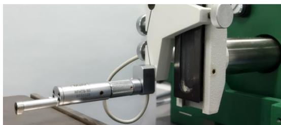
Figure 1. Pick-up and drive unit.
