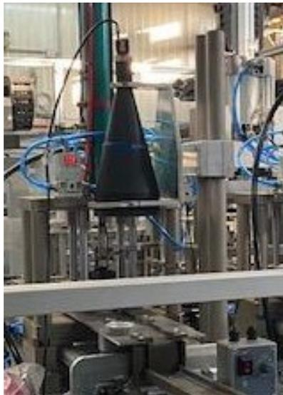
Figure 4. Alvium camera, lens and illumination.
