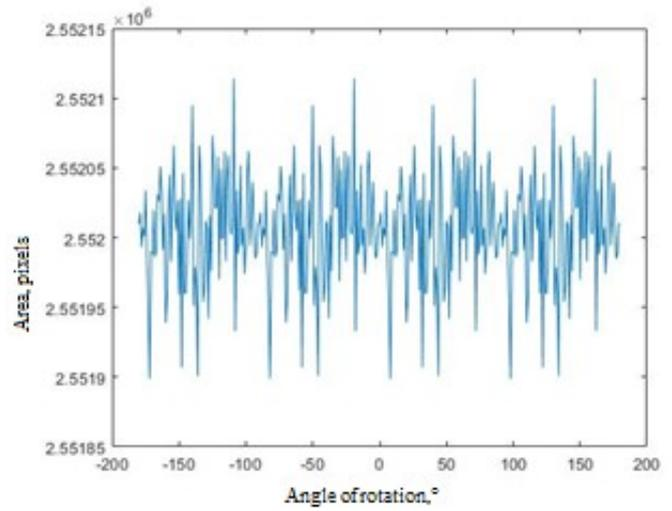
Figure 15. Diagram of the dependence of the number of surface pixels on the angle of rotation for Canon's photo.
