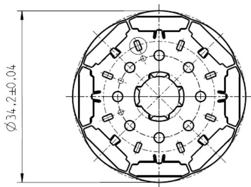
Figure 1. The diameter of the rotor.
