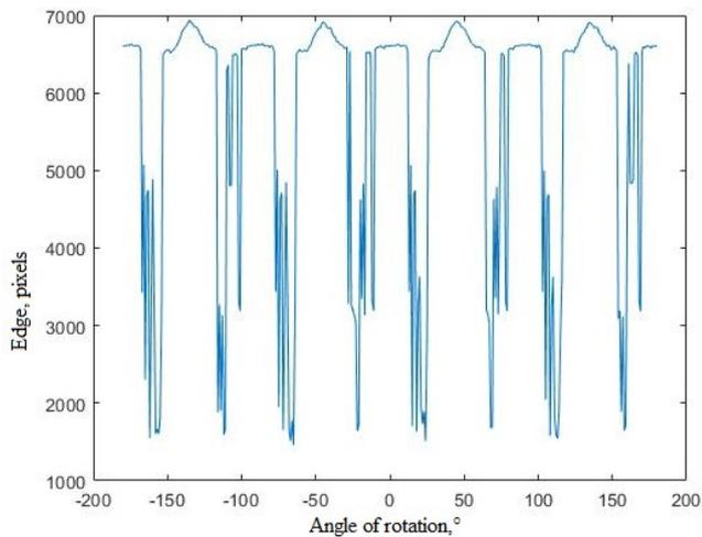
Figure 17. Diagram of the dependence of the number of edge pixels on the angle of rotation for Canon's photo.
