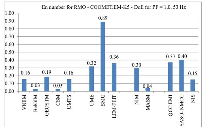
Figure 5.  $E_{ni}$  number for NMI/DI participants of COOMET.EM-K5 KC in the context of RMOs for  $PF = 1.0$  at frequency of 53 Hz.
