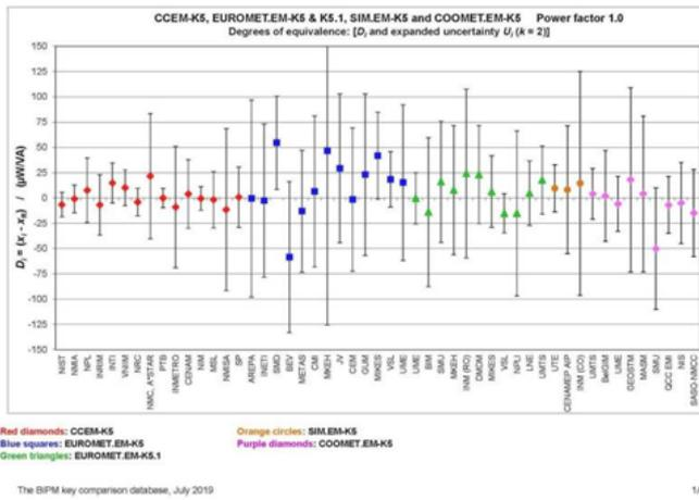
Figure 3. Linked DoE for NMI/DI participants of RMO KCs of power for  $PF = 1.0$  at frequency of 53 Hz.
