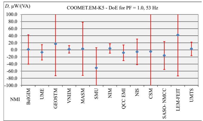
Figure 2. DoE for NMI/DI participants of COOMET.EM-K5 KC for PF = 1.0 0 at frequency of 53 Hz.
