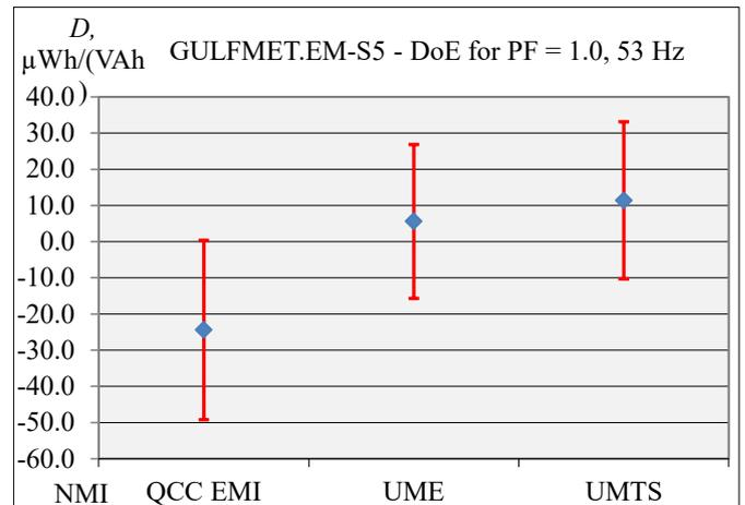
Figure 11. DoE for NMI/DI participants of GULFMET-S5 SC in the context of traceability for  $PF = 1.0$  at frequency of 53 Hz.
