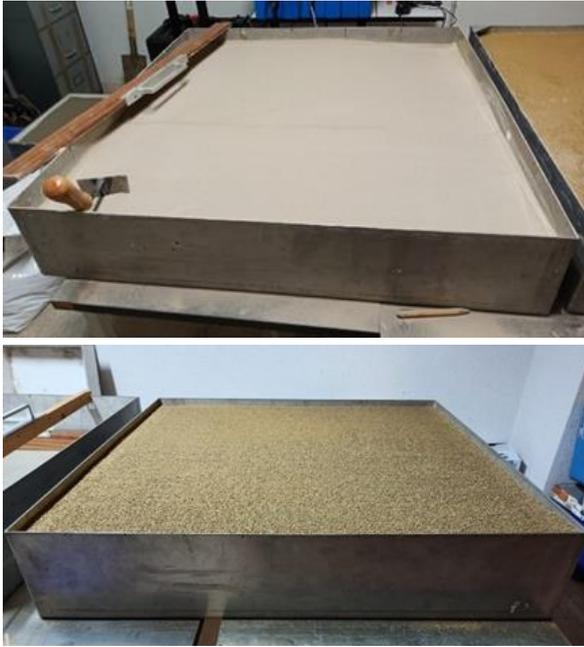
Figure 2. Picture of the Exhalation Beds: Brown, to the bottom: high radon flux, grey, to the top: low radon flux.
