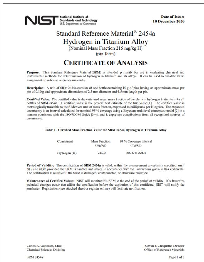
Figure 3. The first page of the certificate for SRM 2454a Hydrogen in Titanium Alloy (Nominal Mass Fraction 215 mg/kg H) (pin form).
