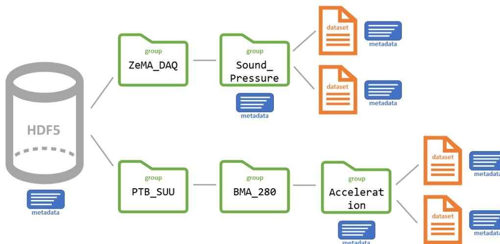
Figure 1. HDF5 file (grey) structure containing groups (green), data sets (orange) and associated metadata (blue).
