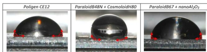
Figure 2. Contact angle measurement of three best performing under UVB aging coatings. Measurements presented here were conducted on non-exposed specimens.
