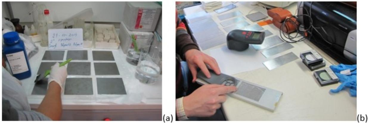
Figure 1. Highlights from laboratory tests during Phase 1: (a) Coating application by brush on uncorroded flat steel specimens and (b) Colour measurements on coated aluminum specimens
