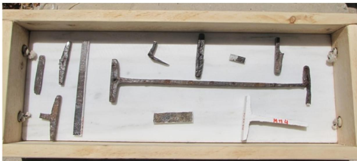
Figure 3. The coated steel joints placed in a marble bottomed open case during field exposure near the monument.
