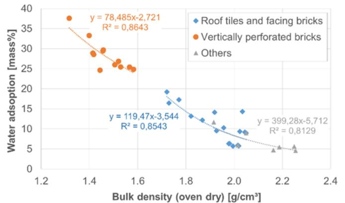
Figure 4. Water adsorption versus bulk density for all samples.
