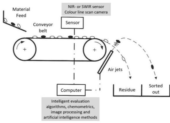
Figure 2. Principle of optical single-grain sorting method.
