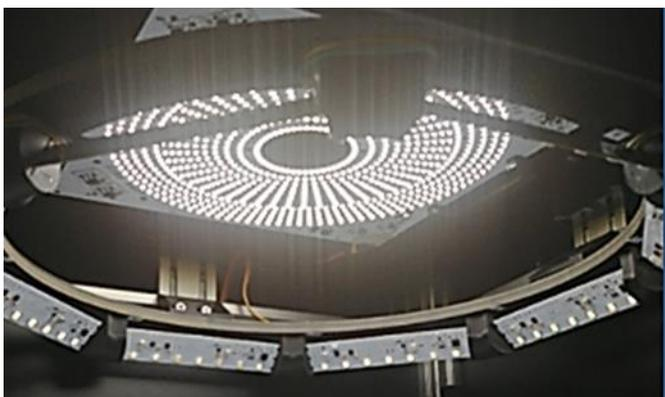
Figure 6. Step-less adjustable lighting system on the QUALILEO.
