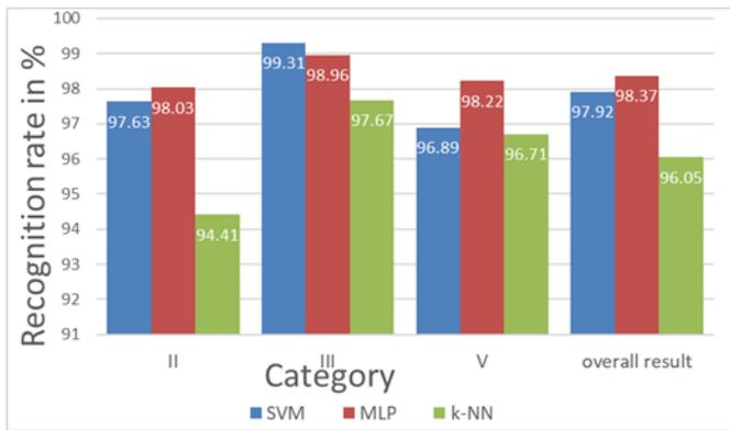
Figure 8. Results of the reached recognition rates for the different brick types using different classifiers on L3 data set.
