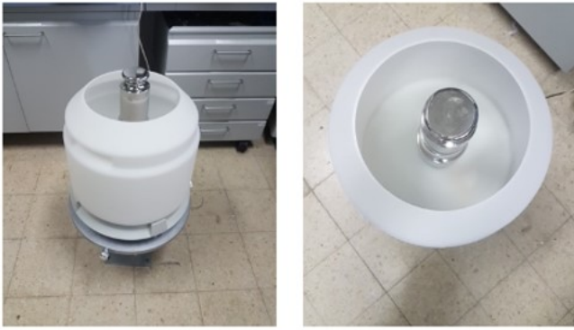
Figure 4. Mass calibration of a rainfall weighing gauge.
