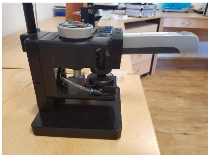
Figure 8. A rebound tonometer on its test bench (detail).
