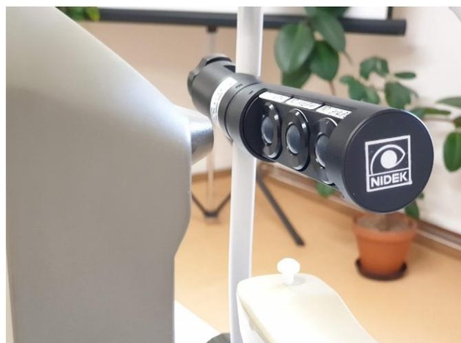
Figure 3. A detail of a non-contact tonometer with a set of the rubber eyes.
