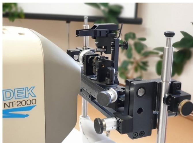
Figure 4. A detail of a non-contact tonometer with a flapper.
