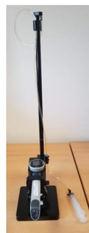
Figure 7. A rebound tonometer on its test bench.
