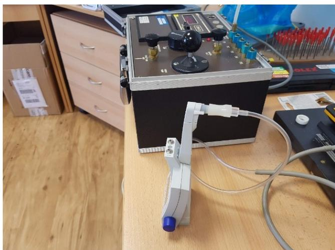
Figure 9. A contour tonometer connected to a pressure standard.
