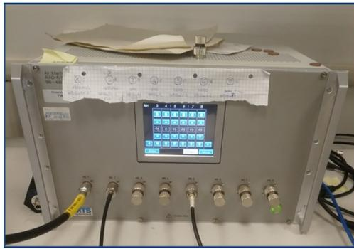
Figure 4. The AIAD used to transfer the signal from the base station to the measurement equipment.
