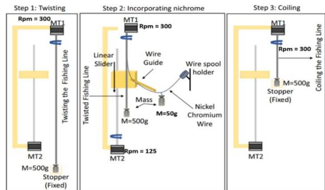
Figure 1. Schematic of the Fabrication process of the Twisted and Coiled Polymer (Fishing Line) muscles. Step1: The Fishing Line Twisting process. Step 2: The Nichrome winding process. Step 3: The Self Coiling process.
