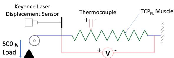
Figure 4. Experimental Setup for the characterization of TCP<sub>FL</sub> muscles.
