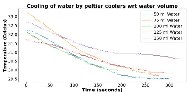
Figure 7. Cooling the water in the housing tank with Peltier coolers. The reduction of temperature in the water was observed over time by the DS18b20 temperature probe for different volumes of water.
