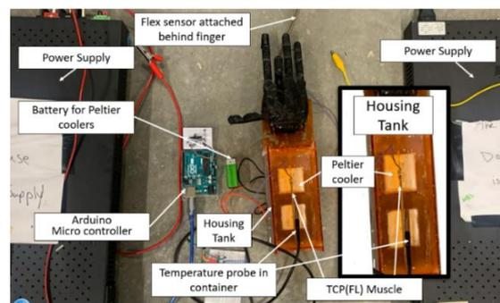
Figure 5. Experimental Setup of TPU hand with TCP<sub>FL</sub> muscles and Peltier Coolers installed housing tank. Two Power supplies used to actuate each of the two muscles for the movement of one finger. The Flex sensor and Temperature probe circuits utilized inside the setup.
