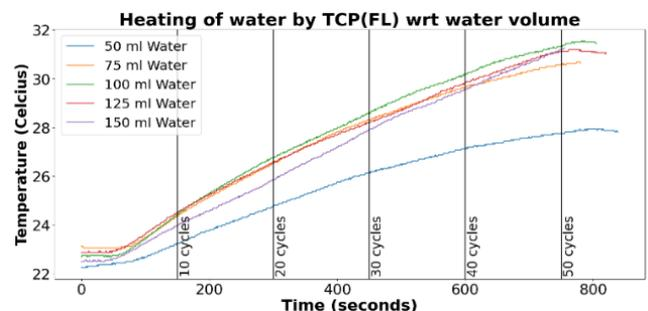
Figure 6. Heating effect of the TCP<sub>FL</sub> muscle actuation on water. The muscle was actuated with a heating cycle of 5 seconds and a cooling cycle of 10 seconds. The steady rise in temperature was observed by the DS18b20 temperature probe over 50 cycles of actuation. The heating effect of the muscle was observed for different volumes of water.
