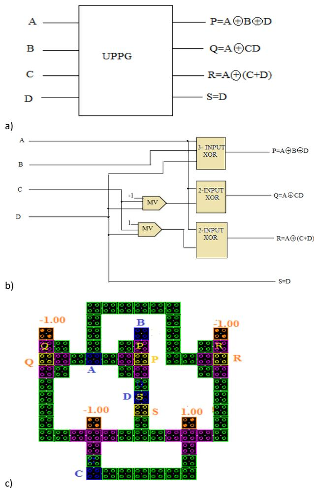
Figure 6. Universal parity preserving gate (UPPG): a) Block diagram, b) Schematic diagram, c) QCA layout.
