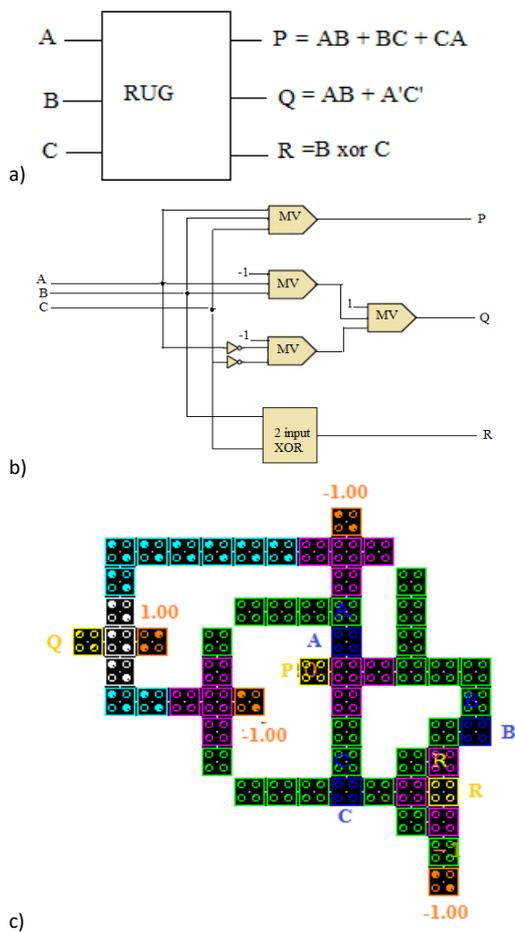
Figure 5. Reversible universal gate (RUG): a) Block diagram, b) Schematic diagram, c) QCA layout.
