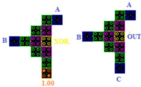
Figure 1. QCA Layout of XOR gate with 2-input and 3-input.
