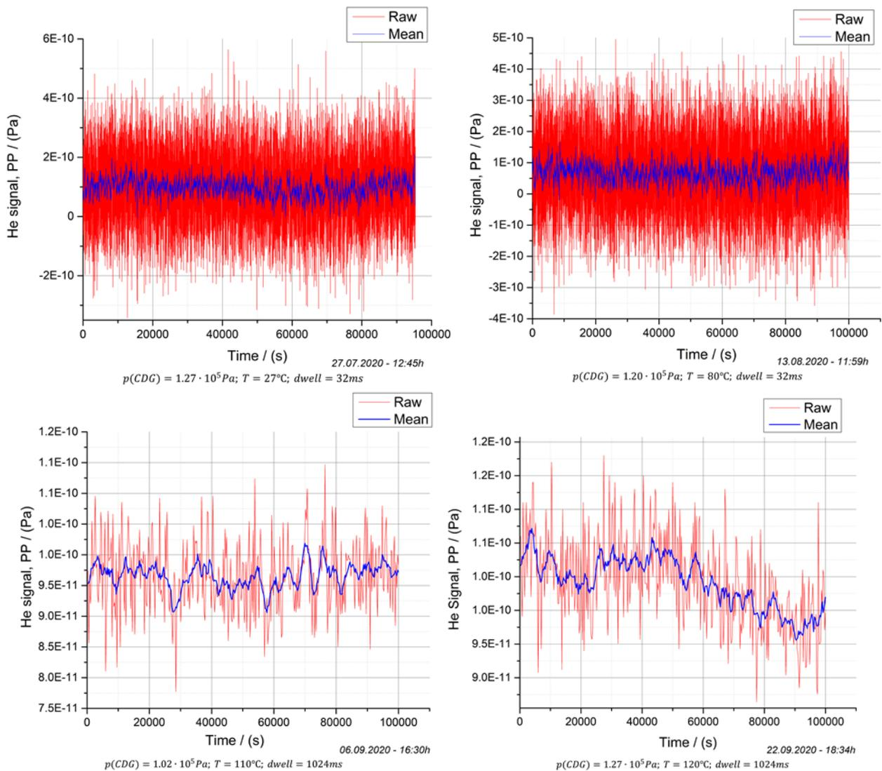
Figure 2. Recorded He signal at different times and temperatures during the study.  $p(\text{CDG})$  indicates the He pressure at the high-pressure volume, measured with the Capacitance Diaphragm Gauge – CDG. In addition to the date of measurements recording, the start time of their registration and dwell time are marked as well.
