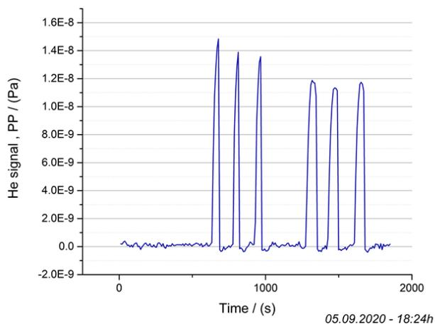
Figure 3. An example of the data conducted with the accumulation method at temperature 110 °C. The first three measurements represent the helium signal recorded by the accumulation method when valve 2 is open while the last three measurements show the helium signal recorded by the accumulation method when valve 2 is closed.
