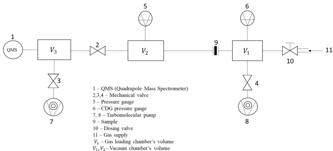
Figure 1. Schematic representation of the vacuum system used to study the permeability of Helium gas into the Zerodur material.
