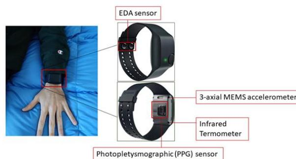
Figure 1. Measurement setup.
