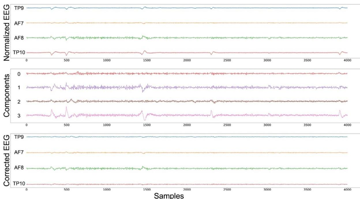
Figure 2. Normalized EEG data before eyeblink component removal; Corrected EEG data after eyeblink component removal and all the components estimated by ICA are reported. Component 3 was rejected.
