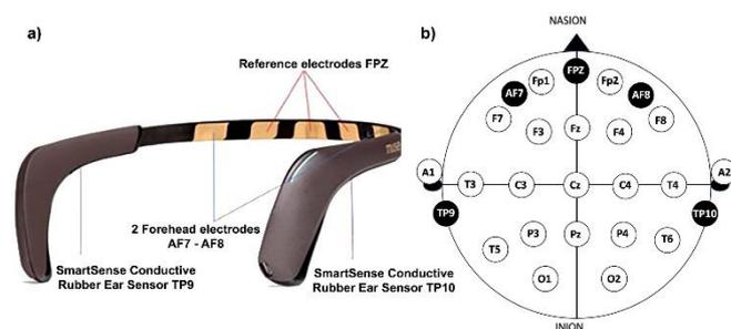
Figure 1. a) MUSE 2 headband sensors overview. b) Top-down view of the EEG electrode positions on the subject's head.
