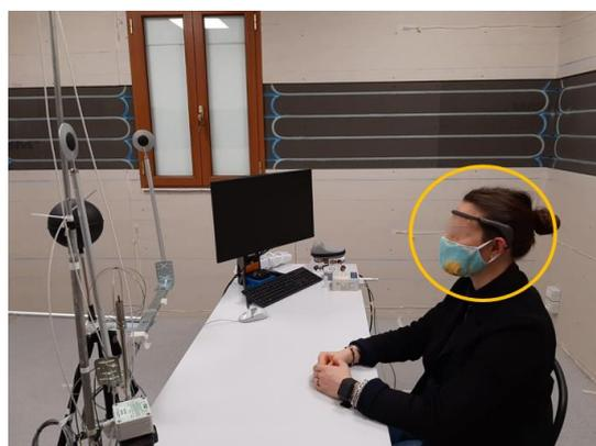
Figure 3. Measurements of EEG signals with Muse headband Interaxon in climate chamber. A facial mask was not used during the experiments.
