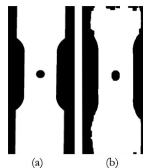
Figure 2. Specimen mask: (a) Visible video (b) Infrared video.
