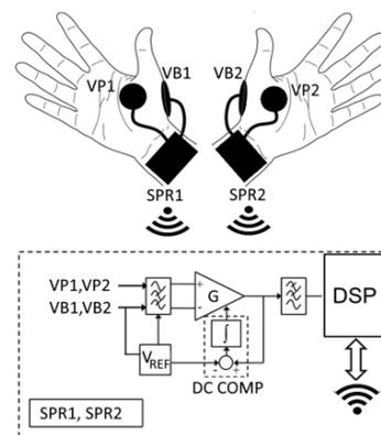
Figure 2. Electrodes arrangement and SPR sensor block diagram.
