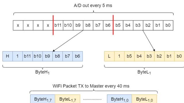
Figure 3. Construction of the packets on the slave for transmission.
