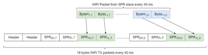
Figure 4. Realignment of the packets on the master.
