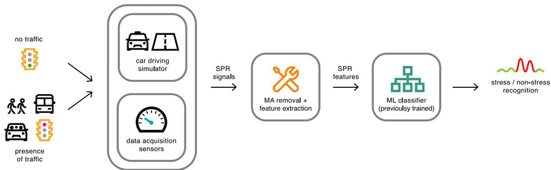
Figure 1. Block scheme of our proposed stress detection measurement system.
