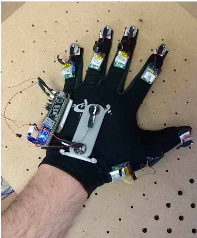
Figure 6. MPS transmitting coils mounted on a wearable glove.
