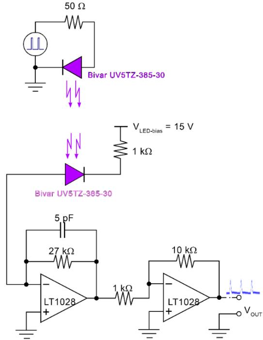
Figure 7. Rx and Tx LED driver circuit.
