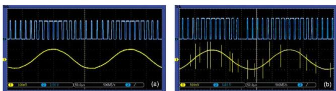
Figure 17. (a) Pulse-width Modulation Waveform. Trace yellow: tone of 4 kHz; trace blue relative PWM modulation. (b) Trace blue: PWM signal recovered in the Rx unit; trace yellow 4 kHz tone present at Rx output.
