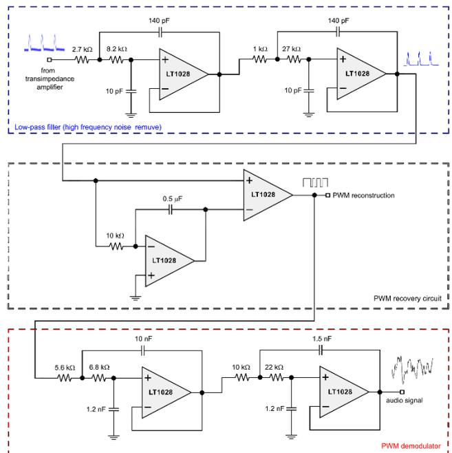
Figure 15. Schematic of the optical receiver circuit.
