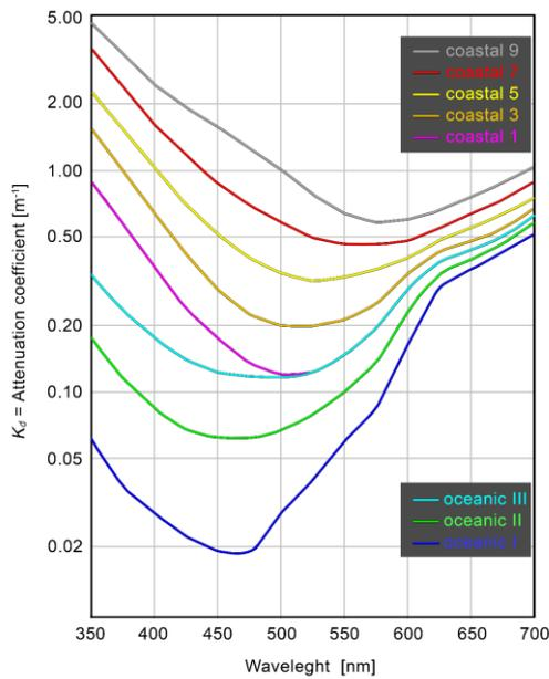
Figure 1. Diffuse attenuation coefficient  $K_d(\lambda)$  for several oceanic and coastal water types according Jerlov classification. Curves obtained from the data present in [9]-[11].
