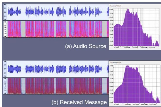
Figure 18. (a) audio track, spectrograms, and frequency analysis of the transmitted audio. (b) audio track, spectrograms, and frequency analysis of the of the retrieved audio signal. Figures obtained by Audacity® software [91].
