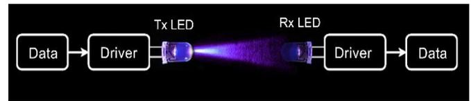
Figure 5. Basic LED used as light emitter and receiver.
