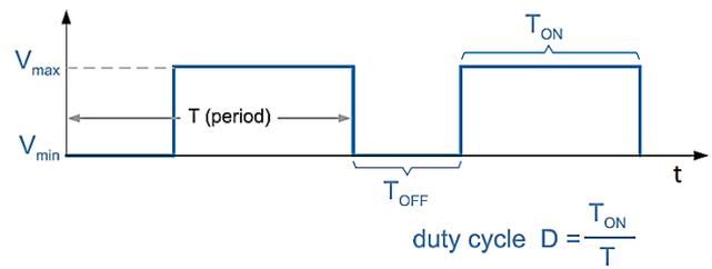
Figure 11. PWM signal. Square wave with constant frequency and amplitude by variable duty cycle.
