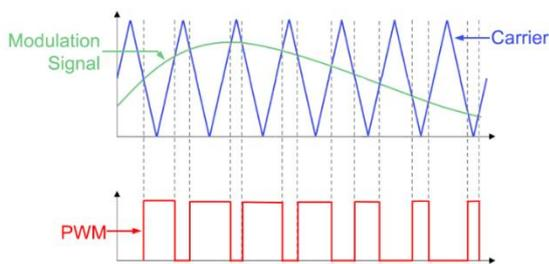
Figure 13. Input and output signals in a Pulse Width Modulation process.
