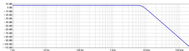
Figure 16. Our 4<sup>th</sup> order Butterworth Low pass filter frequency response.
