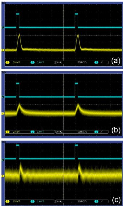
Figure 10. The cyan line represents the signal used to drive the Tx LED. The yellow line represents the corresponding Rx output signal. (a) Distance between transmitter and receiver 0.5 m. (b) Distance between transmitter and receiver 1.5 m. (c) Distance between transmitter and receiver 2.5 m.
