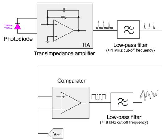
Figure 14. Input and output signals in a Pulse Width Modulation process.
