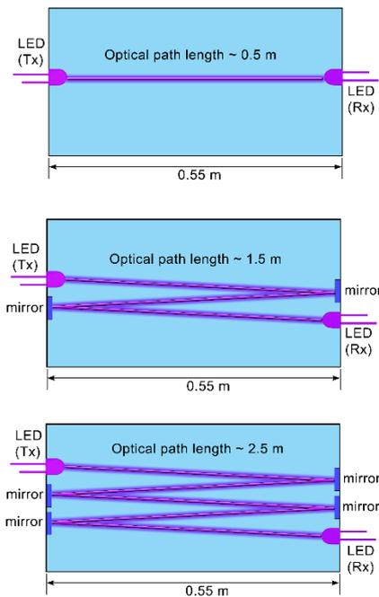
Figure 9. Schematic of the water canal. The different optical path is obtained with the help of mirrors.
