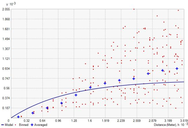
Figure 6. Example of semi-variogram generated for Ordinary kriging application based on the Exponential model.
