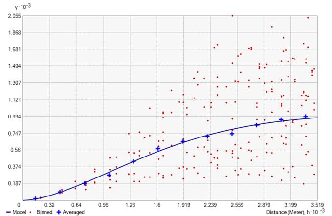
Figure 8. Example of semi-variogram generated for Ordinary kriging application based on the Stable model.
