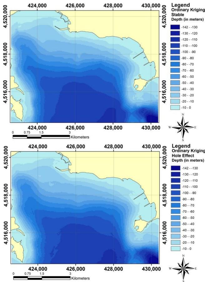
Figure 4. 2D bathymetric models resulting for Ordinary kriging approach from the application of Stable Semi-Variogram Model (top) and Hole Effect Semi-Variogram Model (bottom).
