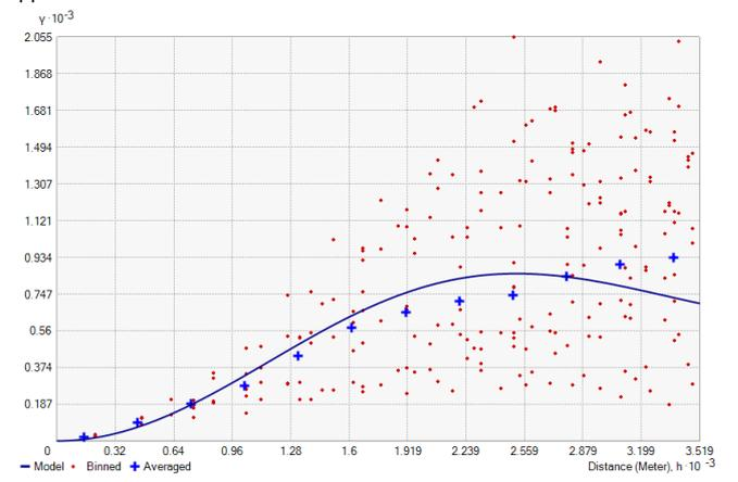
Figure 9. Example of semi-variogram generated for Ordinary kriging application based on the Hole Effect model.
