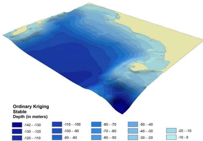
Figure 10. 3D visualization of the most performing bathymetric model generated by Ordinary kriging - STM.
