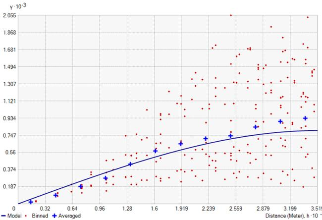
Figure 7. Example of semi-variogram generated for Ordinary kriging application based on the Exponential model.
