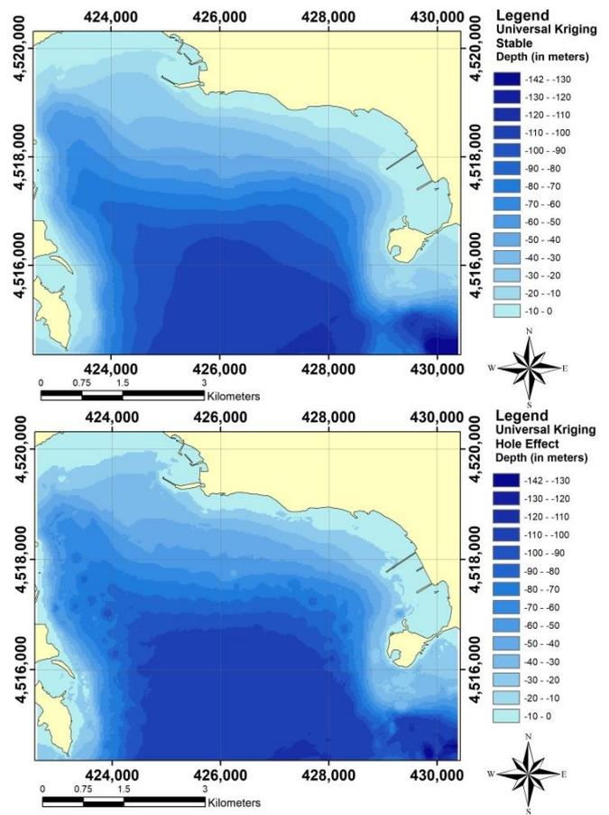
Figure 5. 2D bathymetric models resulting for Universal kriging approach from the application of Stable Semi-Variogram Model (top) and Hole Effect Semi-Variogram Model (bottom).
