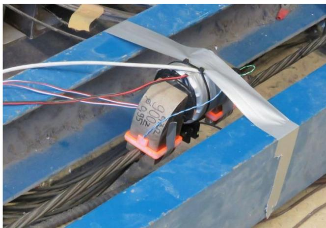
Figure 12. The application of the removable ME sensor on the strand Lp 15.7 in the laboratory conditions
