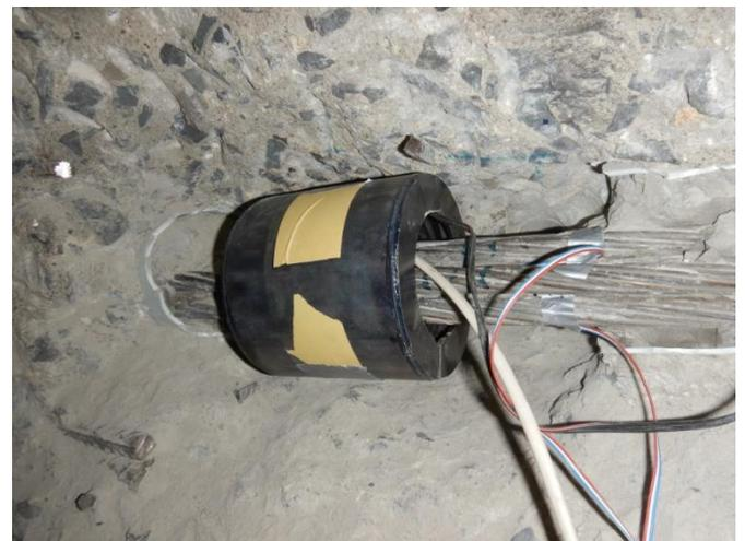
Figure 8. The post installed ME sensor wounded on the prestressed cable composed of twelve strands Lp 15.7 mm
