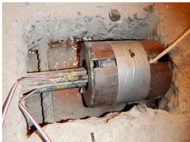
Figure 2. The fully equipped ME sensor installed on the prestressed cable in the inspected bridge
