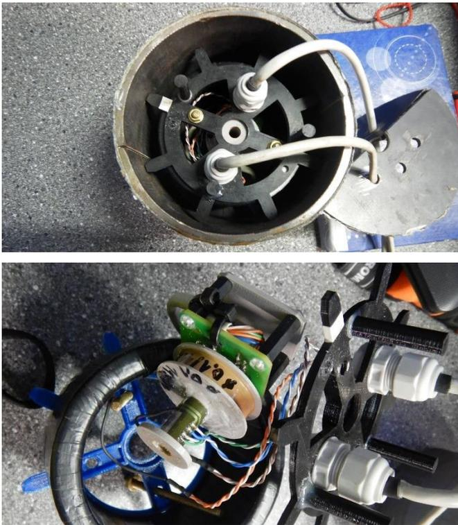
Figure 4. The fully equipped laboratory ME sensor intended for the experiment on the patent wire P7, the assembled sensor inside the steel shield (above) and view on its disassembled basic parts (below)
