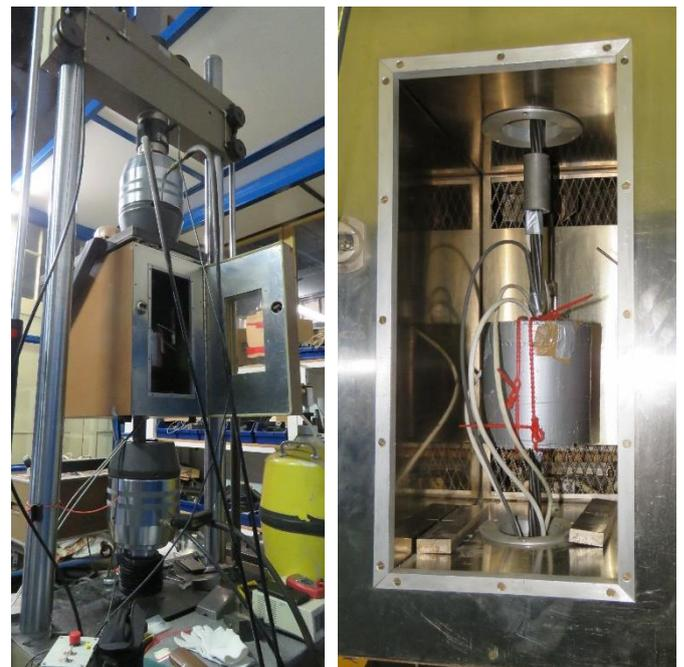
Figure 5. The exterior view on the climatic chamber and the steel tensile testing machine (on the left) and on the laboratory ME sensor installed on the prestressed strand Lp15.7 inside the chamber (on the right)
