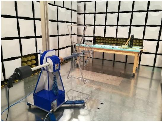
Figure 1. SAC-3 chamber with automotive table and bilog antenna at the University of Miskolc.
