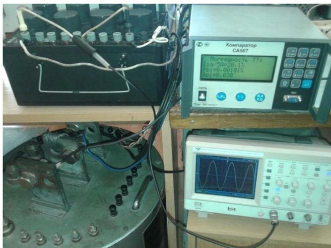
Figure 3. Observation of the shape of the voltage curve at the terminals of the P4834 decade box.
