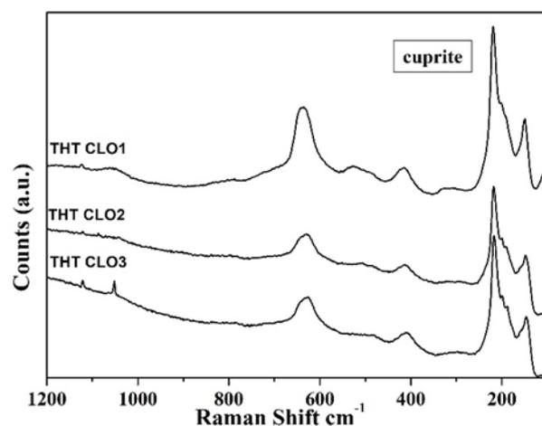
Figure 7. Raman spectra of cuprite (Cu<sub>2</sub>O) on the coins found at Tharros. The Raman spectra collected in a Cu-rich area evidence the presence of poorly crystallised cuprite.
