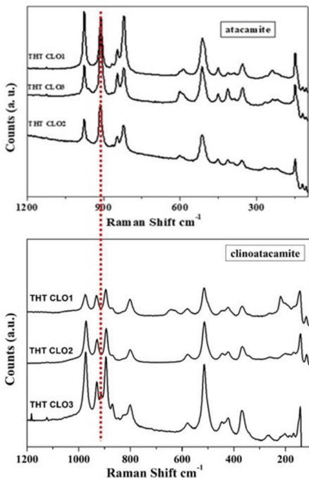
Figure 6. Raman spectra of copper trihydroxychlorides [Cu<sub>2</sub>Cl(OH)<sub>3</sub>] atacamite and clinoatacamite on the coins found at Tharros.
