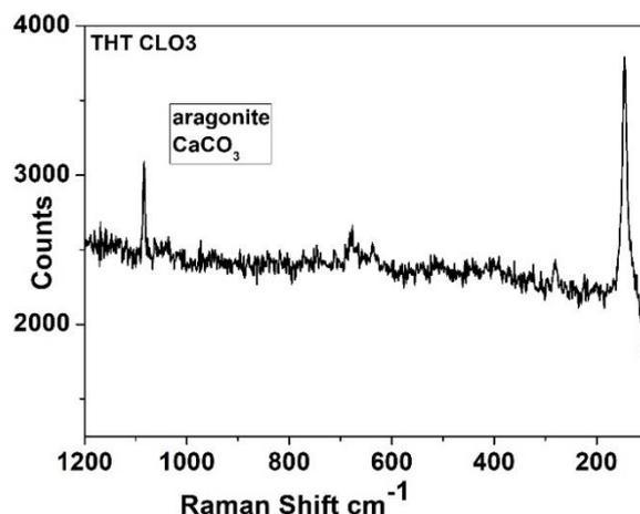
Figure 9. Raman spectrum of aragonite (CaCO<sub>3</sub>) on coin THT CLO3.
