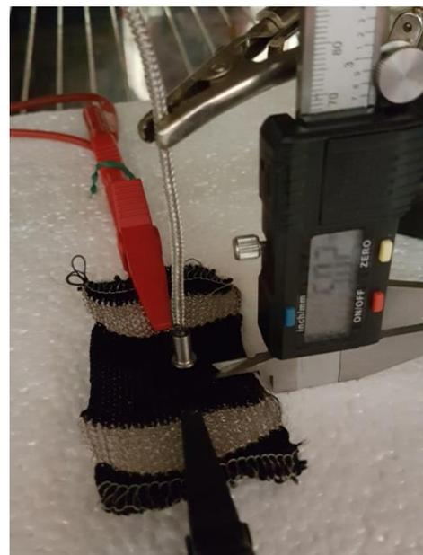
Figure 5. Pt 100 positioned 5mm from sensor.
