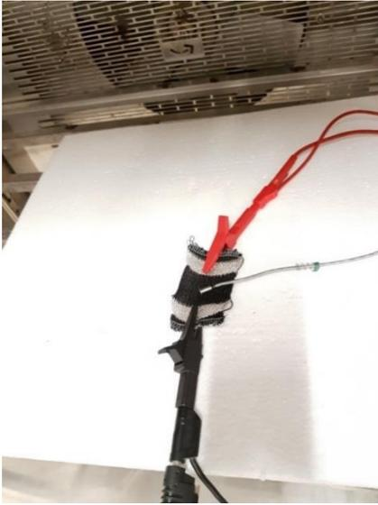
Figure 2. Temperature sensor and Pt100.
