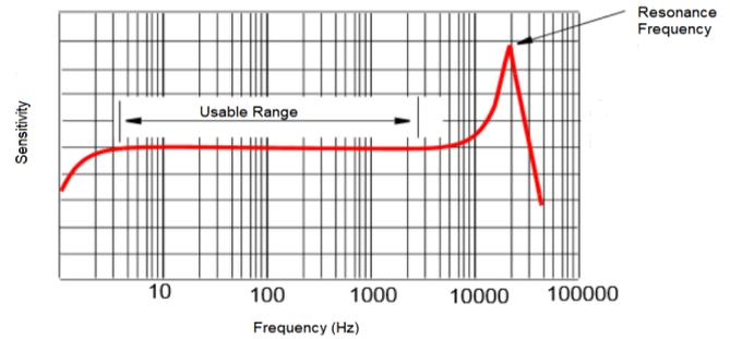
Figure 1. Response-Curve of an Accelerometer
