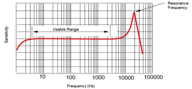
Figure 1. Response-Curve of an Accelerometer
