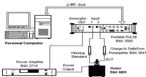
Figure 2. Roketsan Vibration Transducer Calibration System
