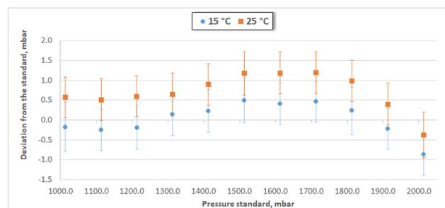
Figure 4: Deviation from the pressure standard at 15 °C and 25 °C
