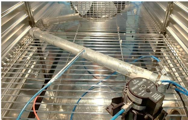
Figure 2: Pressure chamber inside the climatic chamber
