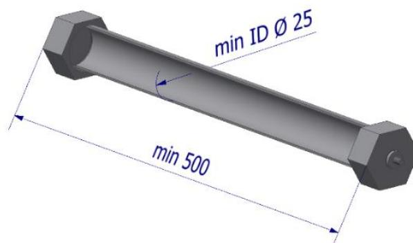
Figure 1: Pressure chamber
