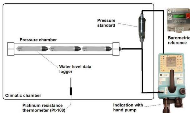
Figure 3: Calibration setup – scheme
