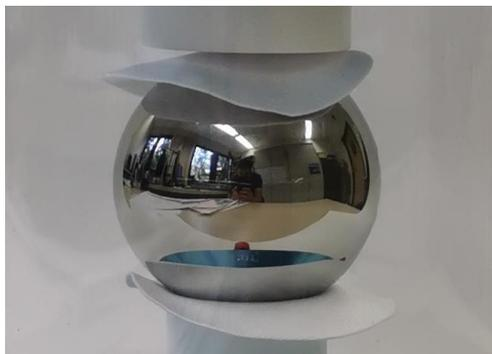
Figure 5: PTB's titanium density standard DS1, owning a nominal volume of 100 cm<sup>3</sup>.
