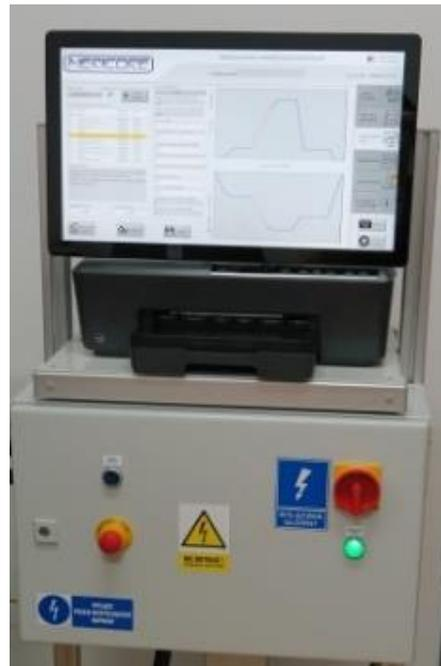
Figure 3: A computer with dedicated software (control and device diagnostics application written in LabVIEW) for data analysis and archiving
